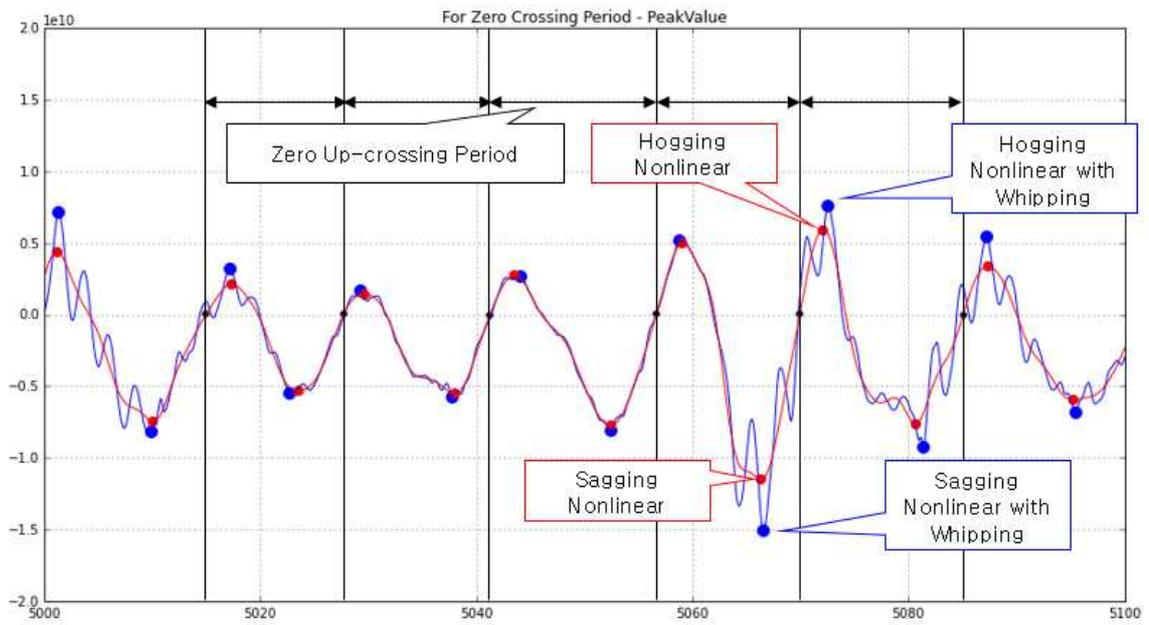
Fig 4.2 Extraction of peak values during load cycle
