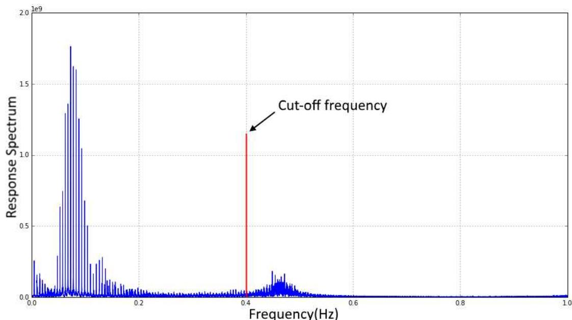
**Fig 4.1 Example of applying cutoff frequency in FFT result of time series data including whipping response**
