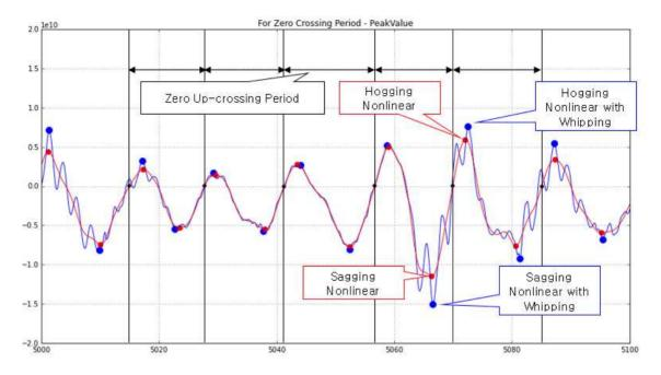
Fig 4.2 Extraction of peak values during load cycle
