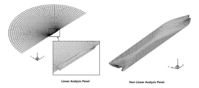
Fig 3.1 Rankine panel model for time domain analysis
