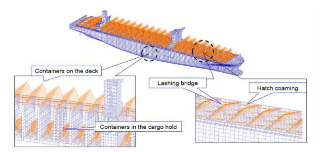
Fig 3.2 Three-dimensional structural model of container ship
