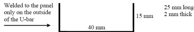
Fig 3.30.1 Welding of U-bar
